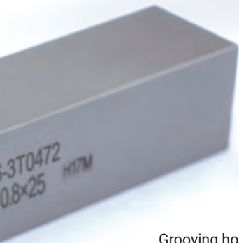
Grooving holder ATSER2525-3T12 and grooving insert ATD302-TS AP301U are used in external grooving of turbine shaft.
